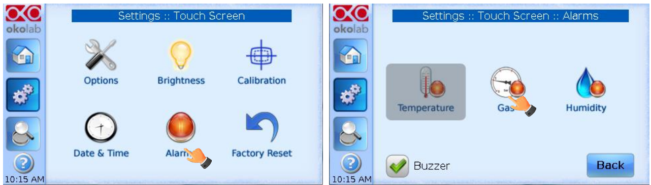
Figure 18. How to enter in Alarms page.
